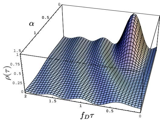
Fig. 6. Crosscorrelation coefficient versus time delay and antenna angle ( $\Delta\omega = 0$ ,  $d_a/\lambda = 1/2$ ).
