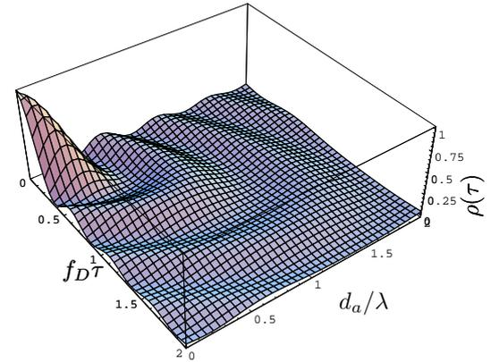
Fig. 5. Crosscorrelation coefficient versus time delay and antenna spacing ( $\Delta\omega = 0$ ,  $\alpha = \pi/4$ ).
