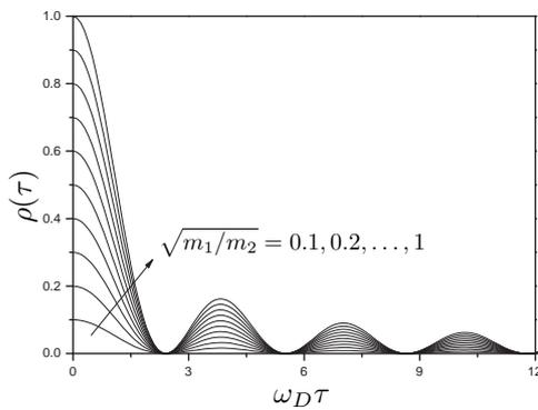
Fig. 4. Crosscorrelation coefficient versus time delay ( $d_a = \Delta\omega = 0$ ).
